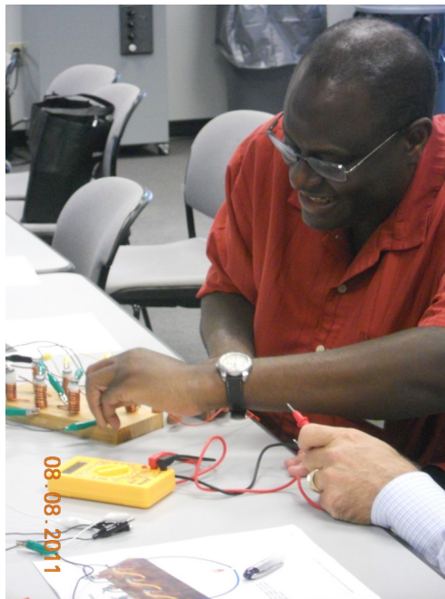
(Below) Tokunbo Ogunfunmi (Santa Clara University) tests the output voltage from the water battery exercise during the Validation/ Verification session.
